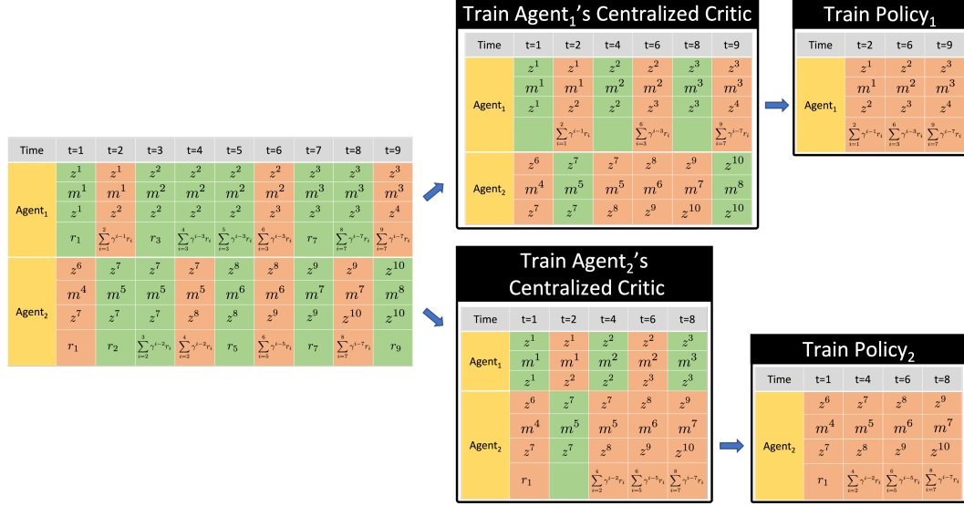
Figure 9: An example of the trajectory squeezing process in Mac-IAICC: each agent learns an individual centralized critic for the decentralized policy optimization. In order to achieve a better use of centralized information, the recurrent layer in each critic’s neural network should receive all the valid joint macro-observation-action information (when any agent terminates its macro-action (line 20-22) and obtain a new joint macro-observation). However, the critic’s TD updates and the policy’s updates still rely on each agent’s individual macro-action termination and the accumulative reward at the corresponding timestep (line 23-26). Hence, the trajectory squeezing process for training each critic still depends on joint-macro-action termination but only retaining the accumulative rewards w.r.t. the corresponding agent’s macro-action termination for computing the TD loss (the middle part in the above picture). Then, each agent’s trajectory is further squeezed depending on its macro-action termination to update the decentralized policy.
